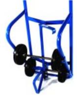
SUPPORT PROP EXTENDS TO STABILIZE THE TRUCK Pushing the chime hook downward extends the prop to hold the truck upright.\* Prop automatically retracts when hook is raised to engage drum rim. Same action used while dispensing.
